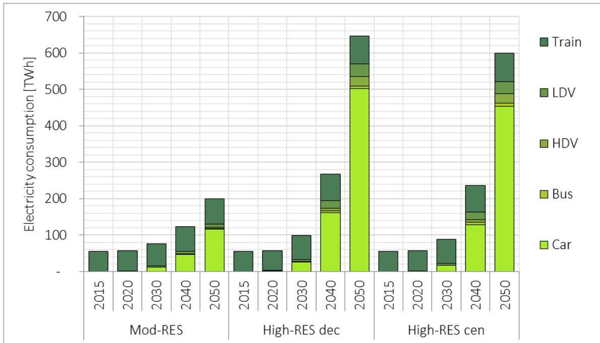
Figure 4: Development of final electricity demand of the transport sector for EU28
