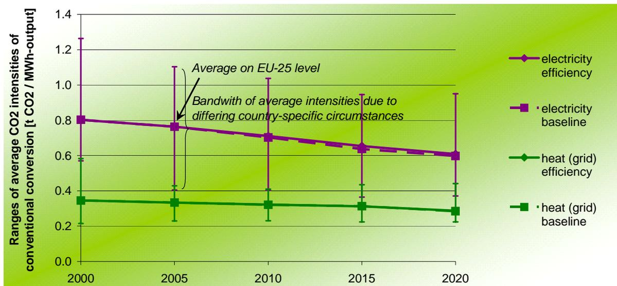
Figure 5 Country-specific average sectoral CO<sub>2</sub> intensities of the conventional (fossil-based) energy system in EU-25 (source: PRIMES scenarios)
